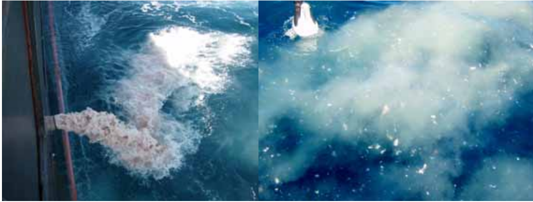
Figure 2 (a) Minced discharge at the outlet (b) Minced discharge in the water. The mince is fine particles, with larger shredded chunks.
