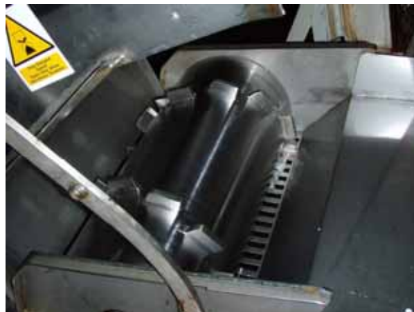
Figure 1 The mincer installed on the vessel
