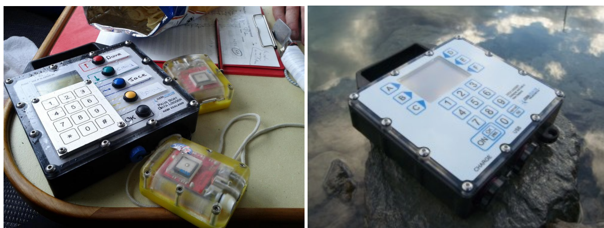
Figure 1: Pāua dive loggers consisting of a boat unit with buttons for recording catch bags and a key pad for entering catch weight and other data, and "turtle loggers" carried by divers (left image). Newly developed deck-logger boat unit (right image; photo courtesy of Zebra-Tech, Nelson).
