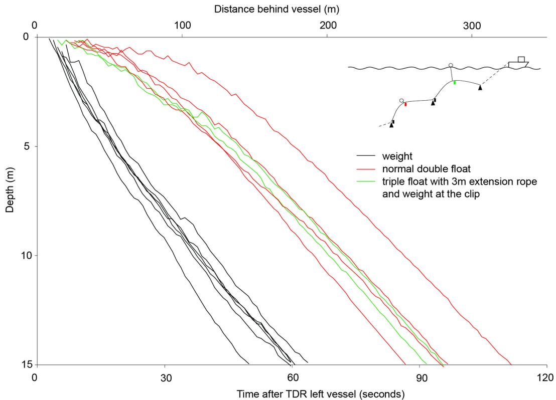
**Figure 20: Time and distance versus depth for time depth recorders (TDRs) deployed on a single line beside weights, floats directly on the line and floats with 3 m rope.**
