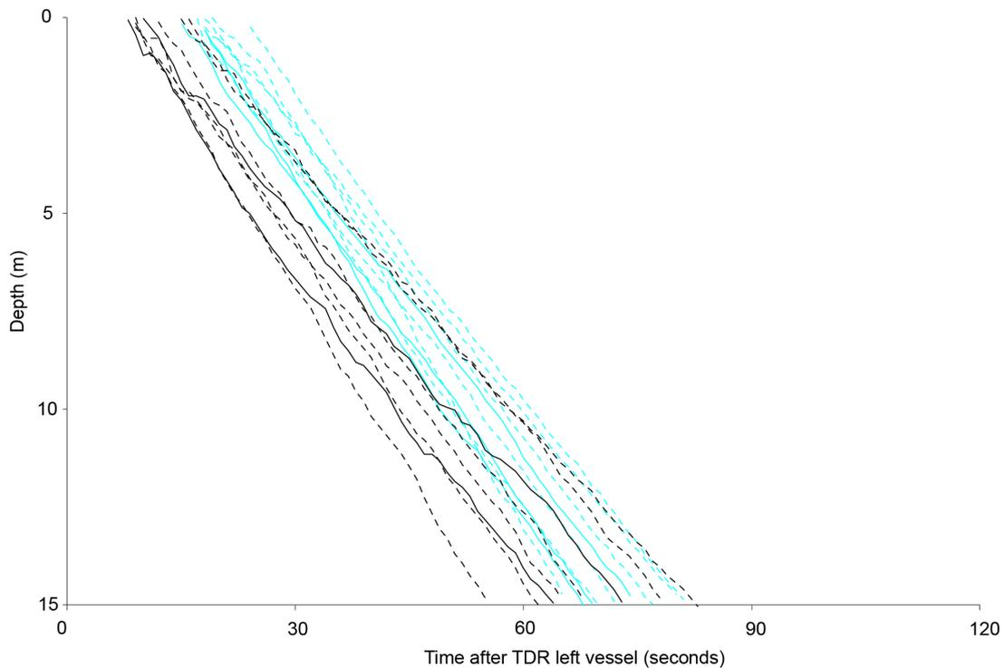
**Figure 16: Plot of time versus depth for TDRs on longlines set at different speeds. Blue lines are from a set at 3.3 knots and black lines from a set at 2.3 knots. Solid lines are from TDRs beside weights and dotted lines between weights.**
