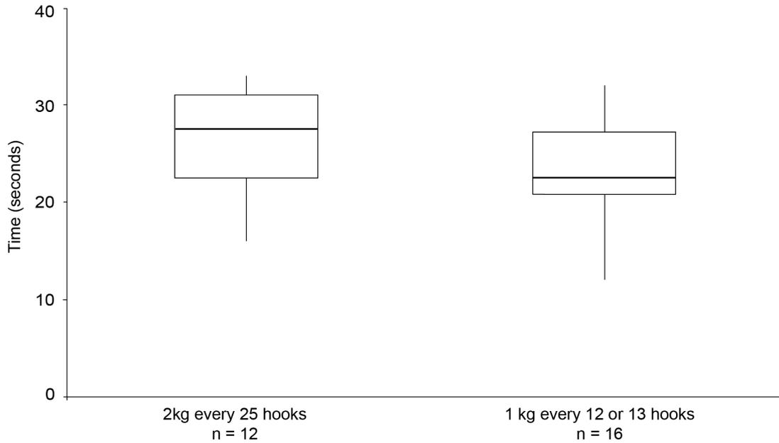
**Figure 17: Box whisker plot of time time depth recorders (TDRs) took to reach 5 m depth with different weighting regimes. TDRs were placed after weights and midway between weights. Three sets were sampled for the normal weighting setup (2 kg every 25 hooks), and two sets were sampled at reduced weight spacing.**
