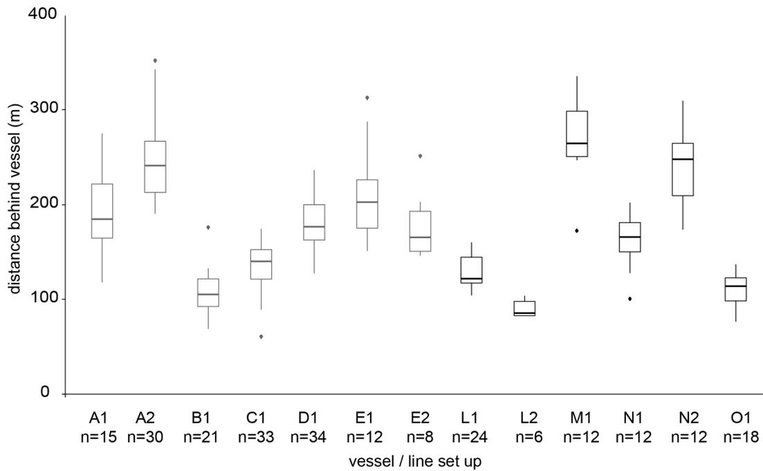
**Figure A-3: Box and whisker plot of distance behind the vessel time depth recorders reached 15 m depth for line setups detailed in Table 10.**
