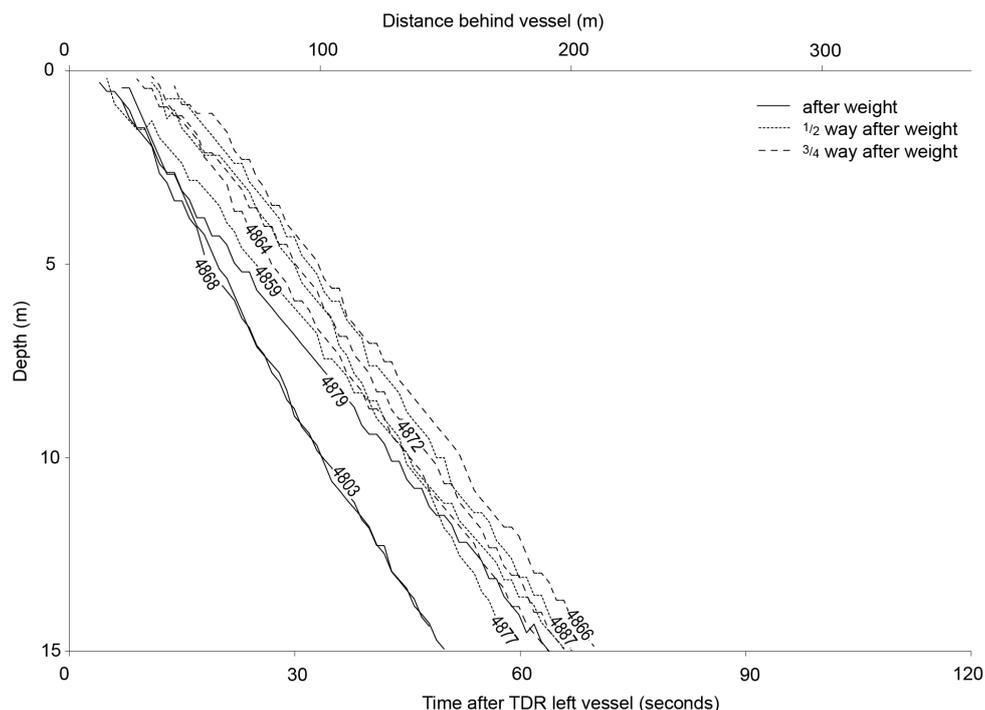
**Figure 9: Time versus depth profiles for time depth recorders (TDRs) deployed during a single set on vessel N, with a repeated line sequence of weight, hooks, weight etc. Individual profiles are labelled with TDR numbers.**
