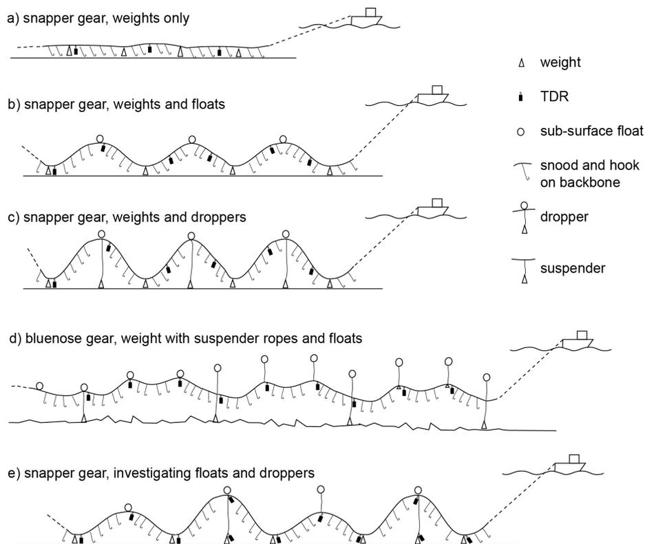
**Figure 1: Position of time-depth recorders (TDRs) on bottom longlines, relative to hooks, weights and floats to investigate sinking rates in snapper (*Pagrus auratus*) and bluenose (*Hyperoglyphe antarctica*) target fisheries.**
