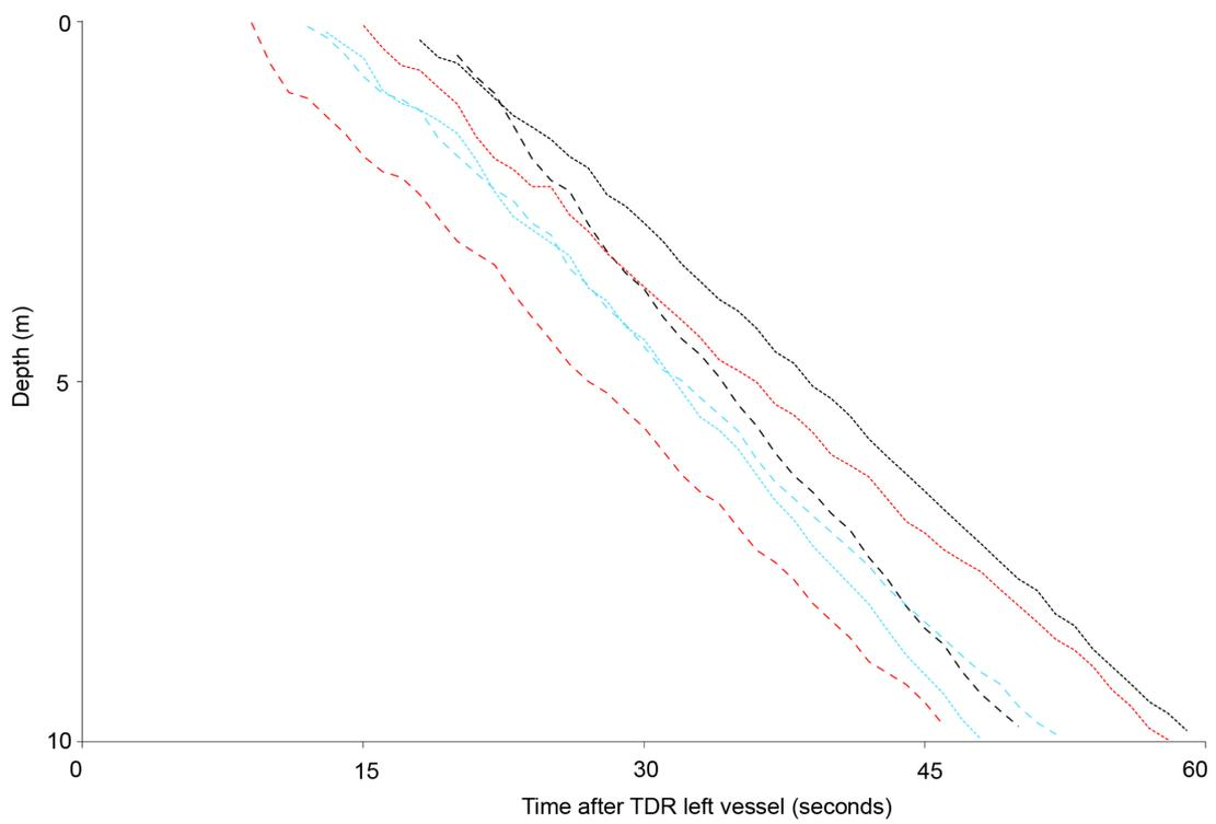
**Figure A-13: Plot of time versus depth for time depth recorders (TDRs) halfway (dotted lines) and three-quarter way (dashed lines) after weights. Consecutive pairs of TDRs are shown in the same colour. Data from vessel O.**
