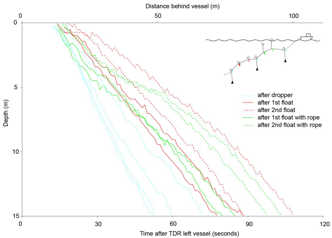
**Figure 23: Time and distance versus depth for time depth recorders (TDRs) deployed on a single line beside weights, floats directly on the line, and floats with a longer rope. Data from vessel Q.**
