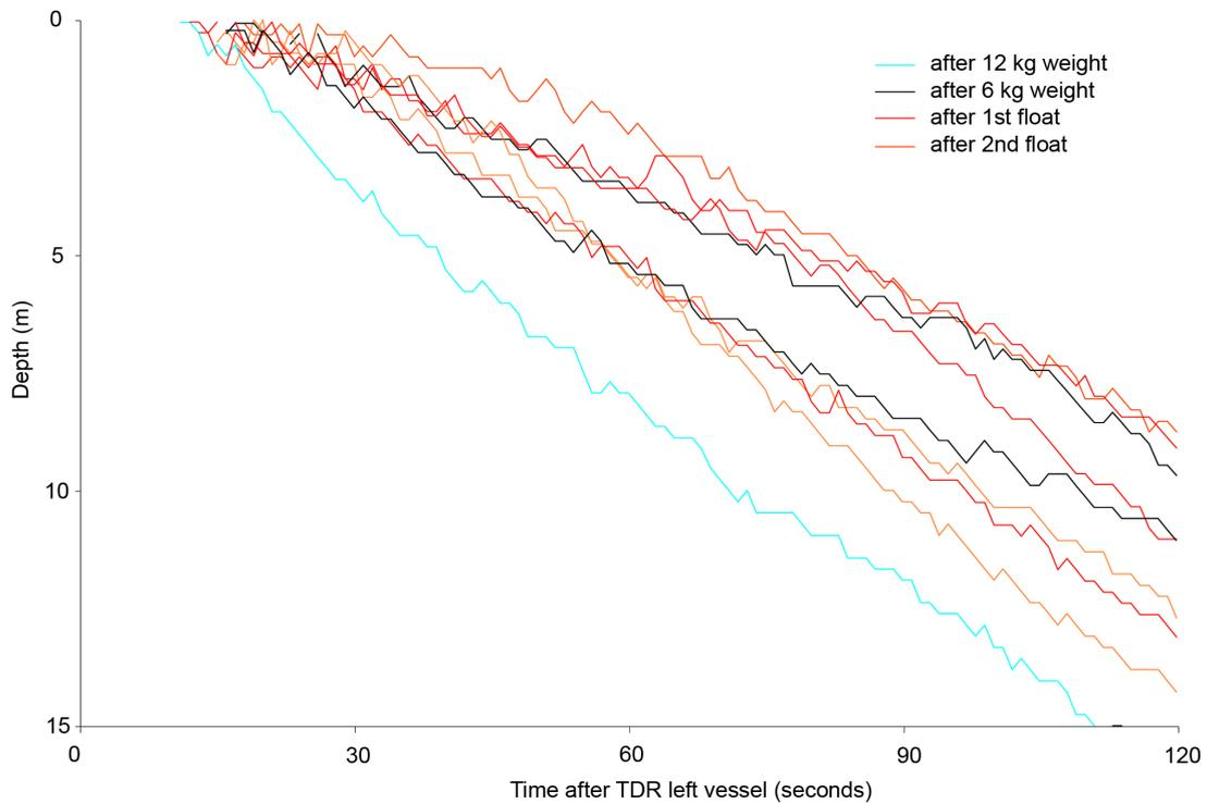
**Figure 15: Time versus depth for time depth recorders (TDRs) placed on three consecutive sections of a line on vessel P. Line setup was weight on a suspender rope, float, float, with every third weight 12 kg rather than 6 kg.**
