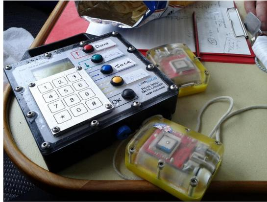
**Figure 1.** Data loggers used in the current study to record catch and effort data in New Zealand’s abalone (pāua, *Haliotis iris*) fishery. The data loggers include a larger boat unit (including buttons for recording catch bags, and a key pad for entering catch weight and other data) and a smaller, dive (or “turtle”) logger that is carried by free divers, and records their position and dive depth (Image by E. Abraham).
