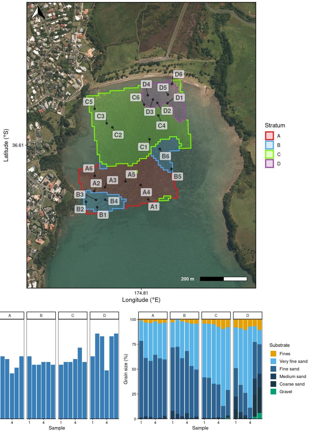
Figure 36: Sediment sample locations and characteristics at Okoromai Bay. Labels correspond to stratum and sample number. Graphs show organic content (% dry weight) and cumulative grain size (%). Sediment grain size fractions include fines (silt and clay, \leq 63 \mu\text{m} ), sands (very fine, >63 \mu\text{m} ; fine, >125 \mu\text{m} ; medium, >250 \mu\text{m} ; coarse, >500 \mu\text{m} ), and gravel ( >2000 \mu\text{m} ) (see details in Table B-1).
