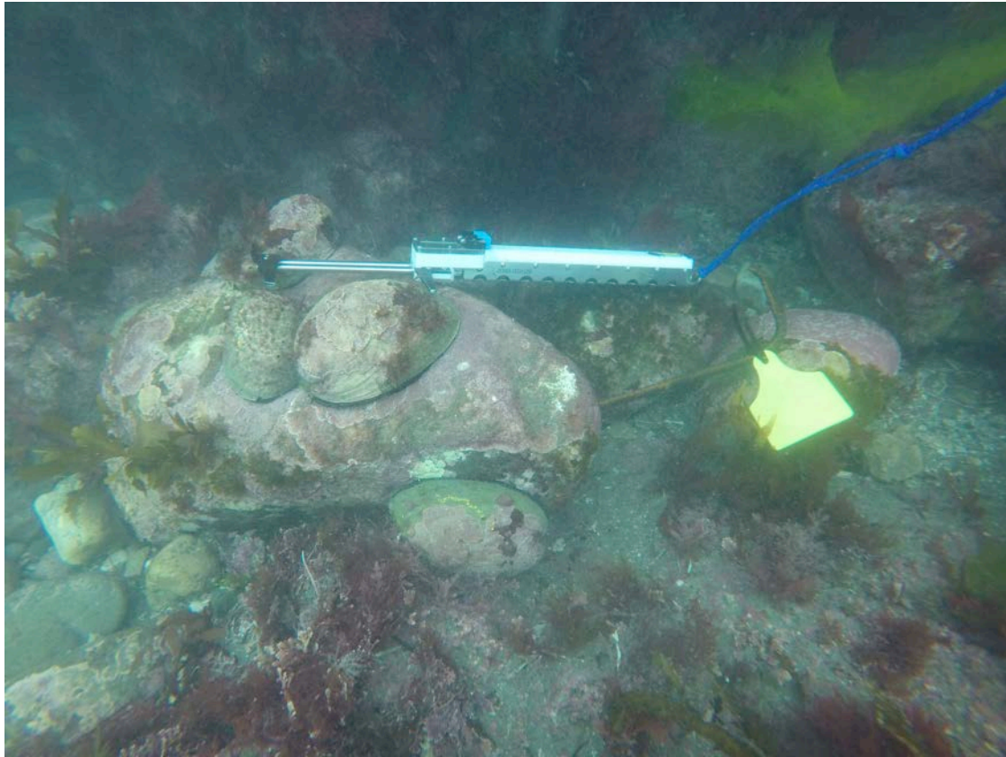
Photograph 1: Monitoring point marked with re-bar and eartag showing underwater electronic callipers used for measuring paua. Note yellow crayon mark on paua indicating that it has been measured.
