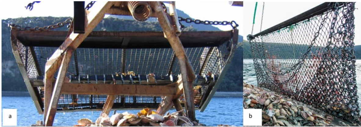
Figure 11: (a) Box dredge and (b) ring-bag dredge used to collect scallops (image sources: J. Williams, NIWA).
