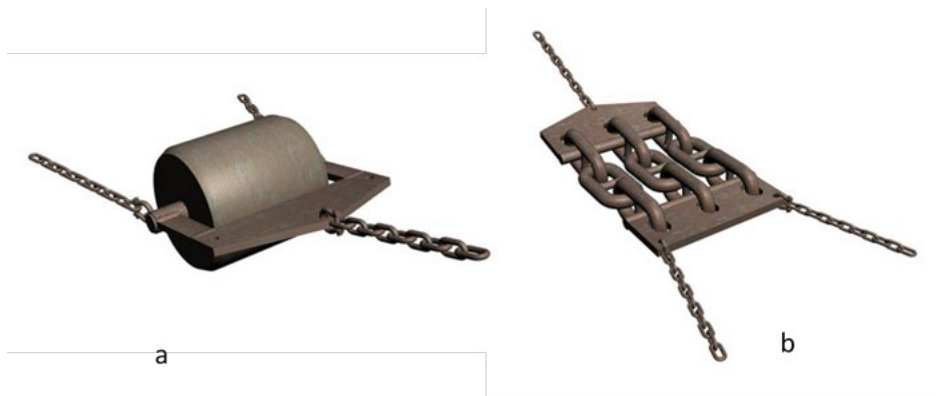
Figure 24: (a) Roller clump and (b) weighted clump which are used as part of bottom gear found on twin-rig trawls (see also Figure 3a. which shows twin-rig arrangement) (image source: with permission from Seafish).
